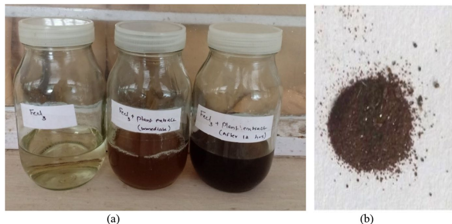
Fig. 1 Formation of PINPs: (a) The figure shows the colorless precursor solution (0.01 M \text{FeCl}_3 ), the solution immediately after mixing precursor and P. korintii leaves aqueous extract (2:3) and the solution obtained 12 h after continuous stirring at 60^\circ\text{C} . The color change of \text{FeCl}_3 solution from colorless to dark brown is the primary indication to the formation of iron nanoparticles (b). The PINPs
